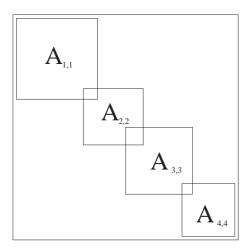
Figure 1. The block Jacobi matrix with overlapping blocks.
