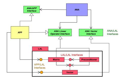
**Figure 1.** UML [6] class diagram : Interfaces between abstract numerical algorithm (ANA), linear algebra library (LAL), and application (APP) software.
