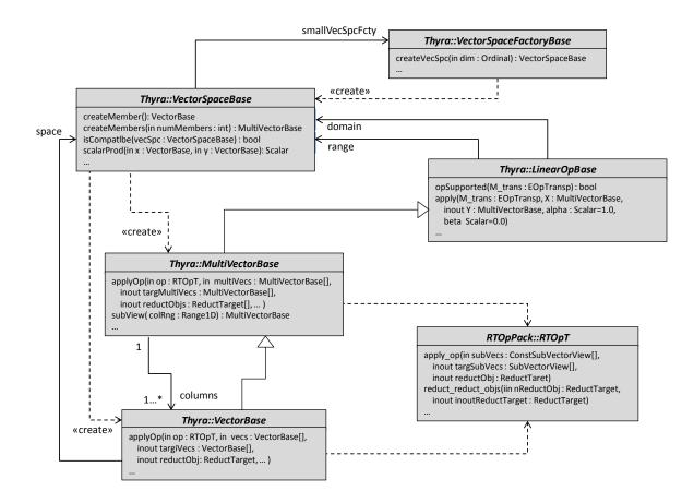
**Figure 2.** UML class diagram : The Thyra fundamental ANA operator/vector interfaces
